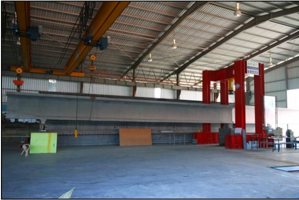
Full scale flexure strength test for TBG1325-29.5m.
