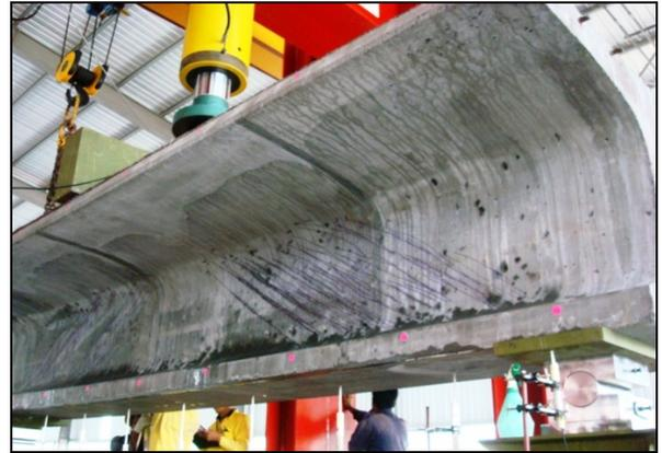
Full scale shear strength test for TBG875-8m
